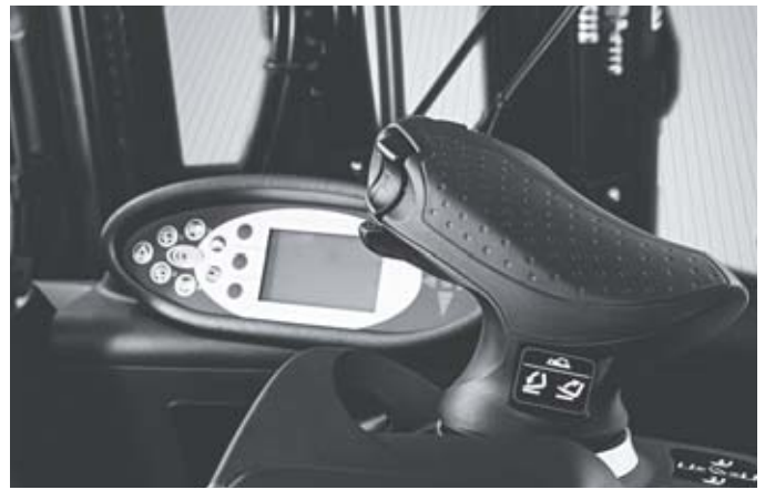
Convenient and precise hydraulic operation with Joystick 4Plus
