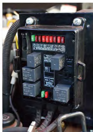
Modular high protection electrical box
